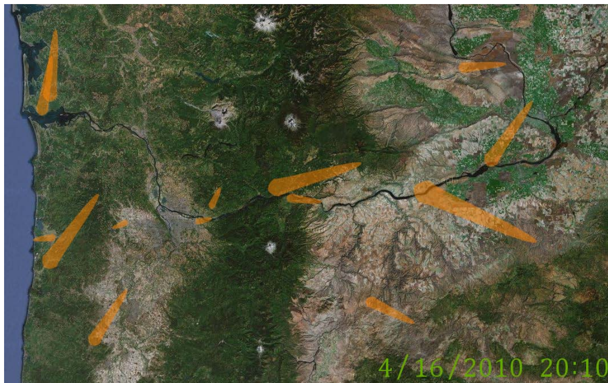
Figure 14: BPA's Windsock Display shows the system operator wind speed and direction to help forecast output from the region's wind fleet.
